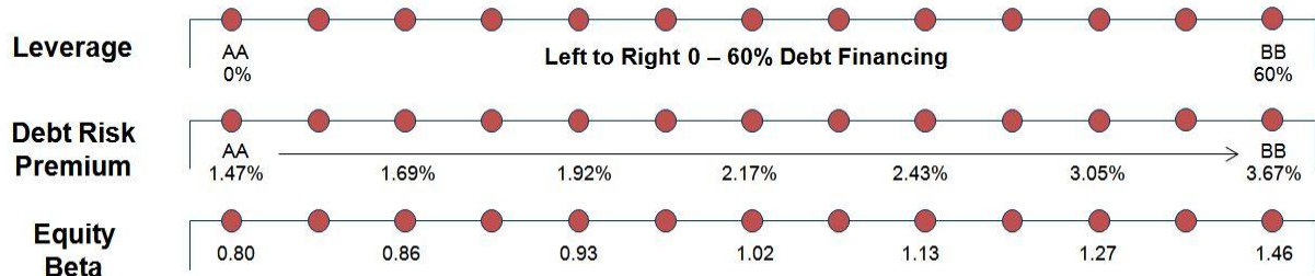
Figure 4 Example mapping from gearing (D/V) to debt risk premium and equity beta. The credit ratings at the end points are dependent on the qualitative risk assessment of the port ascertained from the Moody's survey.
