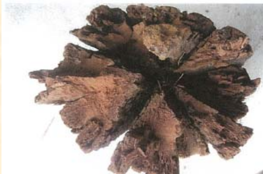
Picture 1. Pole PID# 338949 showing the extent of the rot and five separate sections.
